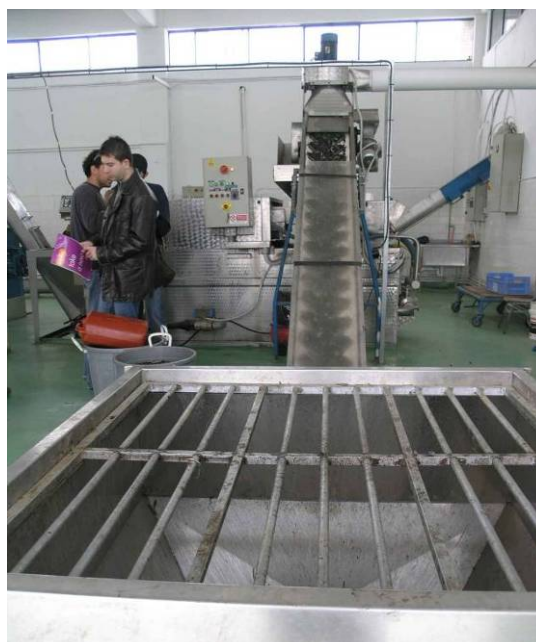
Figure 30 – Olives elevated from crate to suction and washing machine
