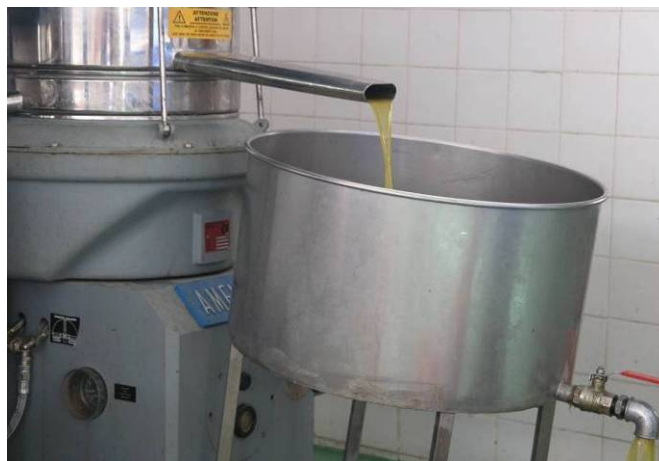
Figure 37 – Oil separation in Lythrodontas
